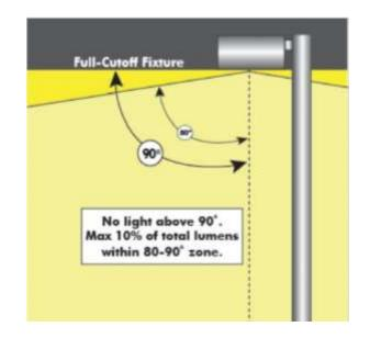
*Full cutoff fixtures do not allow any light to be emitted above the fixture. The fixture controls glare by limiting the light output at 10 degress below the horizontal.*
